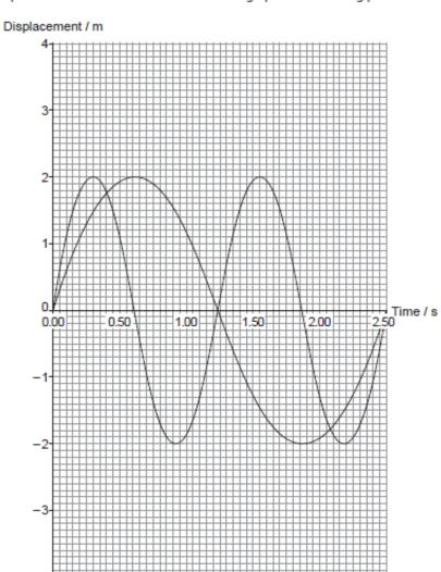
Use the principle of superposition to plot the resultant displacement of the two waves at times 0.00s, 0.40s, 1.00s, 1.25s, 1.50s, 2.10s, 2.50s on the same grid and draw a suitable curve. [4]
